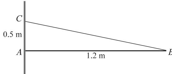
A uniform rod  $AB$  of length 1.2 m and weight 30 N is in equilibrium with the end  $A$  in contact with a vertical wall.  $AB$  is held at right angles to the wall by a light inextensible string. The string has one end attached to the rod at  $B$  and the other end attached to a point  $C$  of the wall. The point  $C$  is 0.5 m vertically above  $A$  (see diagram). Find
