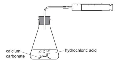
The volume of gas in the syringe is recorded after one minute.
