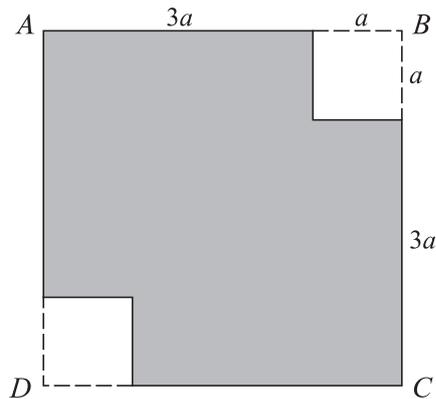
A uniform square plate  $ABCD$ , of side  $4a$  and mass  $M$ , has squares of side  $a$  cut from the corners at  $B$  and  $D$  (see diagram). Show that the moment of inertia of the resulting lamina about an axis through  $A$  and perpendicular to the plane of the lamina is  $\frac{109}{12}Ma^2$ . [8]
