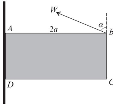
A uniform rectangular lamina  $ABCD$  has  $AB = 2a$  and weight  $W$ . It is supported with  $AD$  in contact with a rough vertical wall. The lamina is in a vertical plane perpendicular to the wall and is held in equilibrium by a force of magnitude  $W$  acting at  $B$ . This force acts at an angle  $\alpha$  to the vertical and in the plane of the lamina (see diagram). The coefficient of friction between the lamina and the wall is  $\mu$ . Show that  $\mu \geq \tan \frac{1}{2}\alpha$ . [7]
