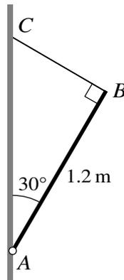
A non-uniform rod  $AB$  of mass 2 kg and of length 1.2 m is smoothly hinged at  $A$  in a vertical plane perpendicular to a vertical wall. The rod is kept in equilibrium by a light inextensible string attached to  $B$  and to the wall at  $C$ , vertically above  $A$ , where angle  $ABC = 90^\circ$  and angle  $CAB = 30^\circ$  (see diagram). The tension in the string is 7.5 N.
